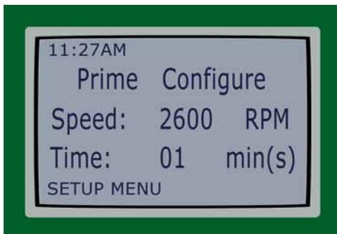
The priming speed and time can be adjusted within this menu. The minimum priming speed is 1500 RPM. The maximum priming time is 10 minutes.
