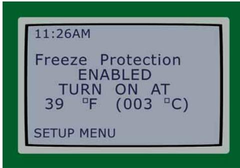
Freeze Protection can be either enabled or disabled when the user turns the User Interface selector knob to Setup. If it is enabled, the user will be able to set the temperature at which the pump will turn on. The control is designed to run the pump for 8 hours at 2600 RPM if the temperature drops below the setpoint.
