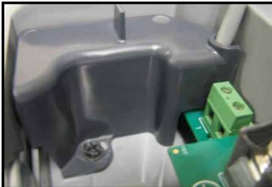
**Figure 15: Plastic Cover Installed In Terminal Box**
